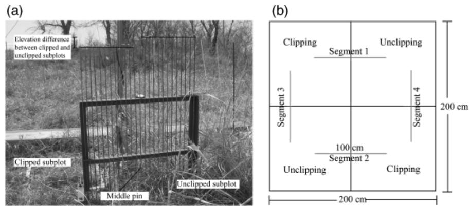
Fig. 1 Self-made apparatus for measuring the relative erosion depth in this study (a), and the placement of apparatus in each plot (b).
