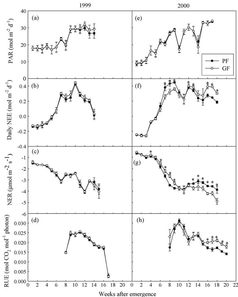
**Fig. 3.** The weekly averaged PAR levels, daily NEE, NER and canopy RUE<sub>CO<sub>2</sub></sub> in two EcoCELLs in 1999 (a–d) vs. 2000 (e–h). The error bars represent the standard error of the weekly mean. “\*” indicates significant difference between PF and GF at the level of  $p < 0.05$  ( $t$ -test).
