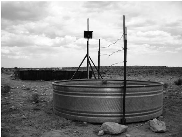
Figure 1. Experimental trough design at Raymond Wildlife Area, Arizona, USA, showing a modified circular and an unmodified rectangular trough (1 Jul 2004). Black and white video cameras and infrared lights are mounted on the pole between the troughs. The recording equipment is located 76 m away from the troughs.
